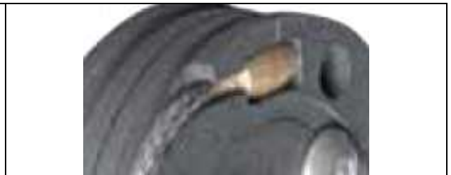
Fig. 31 : assembled drive wire in a tensionable drive wheel
