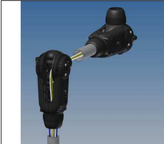
Fig. 34: Two wire pairs are fed through the lower joint
