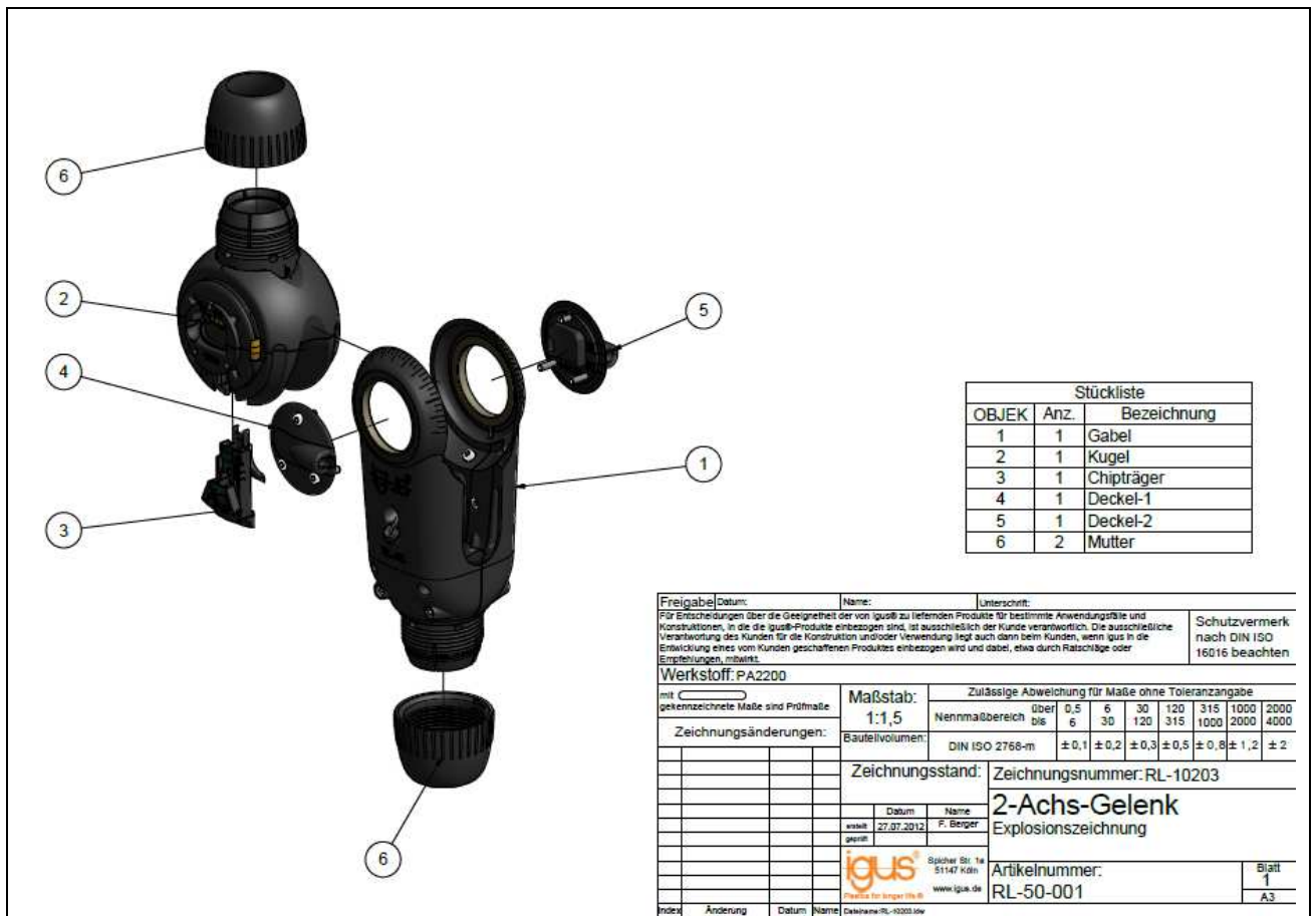
Fig. 55: Exploded drawing / parts list - 2 axes joint RL-50-001 (-002)
