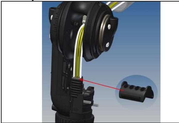
Fig. 36: Bowden cable segments for parallel feed-through
